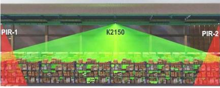
✤ If the height of the warehouse does not exceed 14m, they use a scheme with two sensors (PIR) – at the beginning and at the end of the alley + a long time delay (usually 10 minutes)
