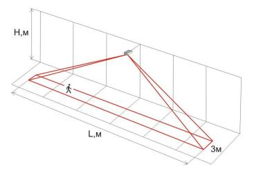
The length of the K2150 sensor's sensitive area depends on the installation height H (person's movement tracing!).
