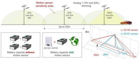
K2150 motion sensor reduces the battery capacity by several times!
