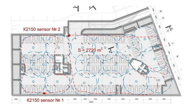
Two K2150 sensors instead of 17 ceiling PIR sensors in underground **car parking lot.**
